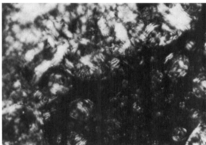
FIGURE 9 Liquid crystal behavior of PGLU(pTFMB), at 25°C, in tetrahydrofuran solvent showing an early stage of the biphasic region under the polarizing microscope. The small liquid crystal domains that are present appear to be less uniform and regular than for the other polymers. See Color Plate VIII.
